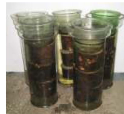
20-sm bolts of Siberian fir submerged in buckets with cold water for 1 to 4 weeks (3 bolts for each treatment).
